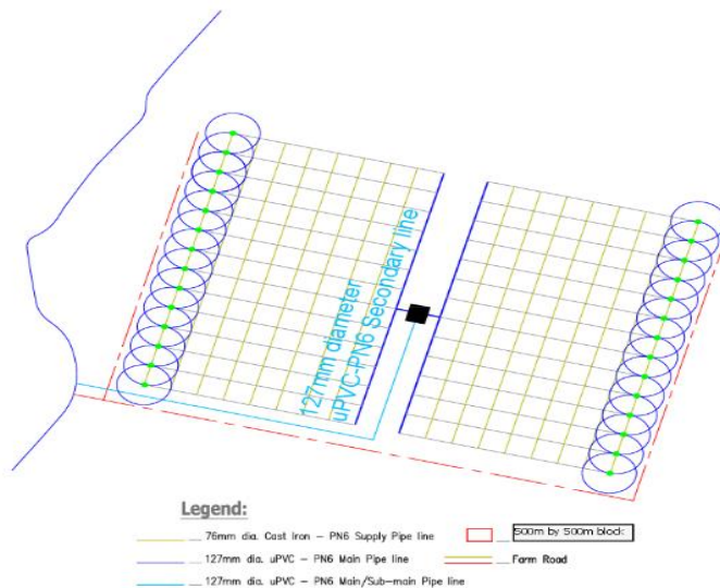
Fig. 2. Semi-Solid Set Sprinkler Irrigation System at Mkulazi Sugarcane Estate
