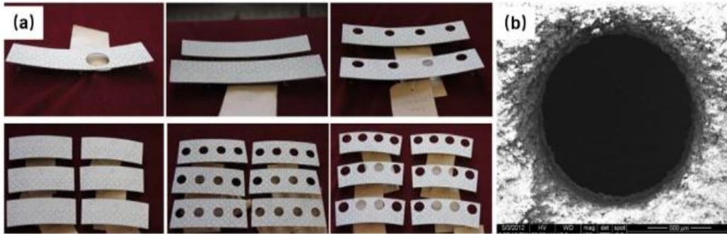
Fig. 10. (a) TBCs coated on the combustor tile and (b) the edge morphology of the cooling hole with TBCs
