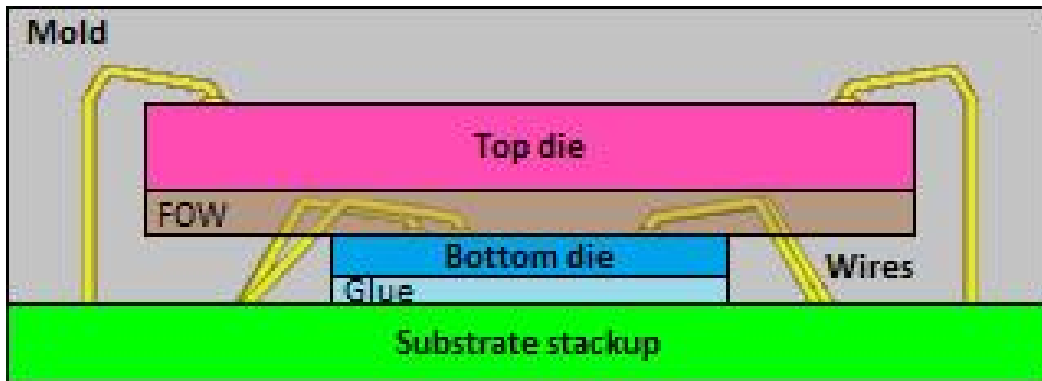
Fig. 1. Multi-die package design cross-section
